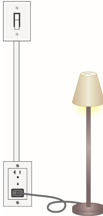
Where a switch controls a receptacle load
